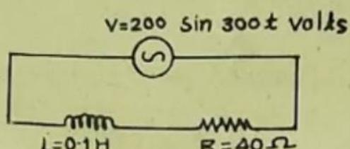
In the following alternating current circuit, find the current and power factor of the circuit.
